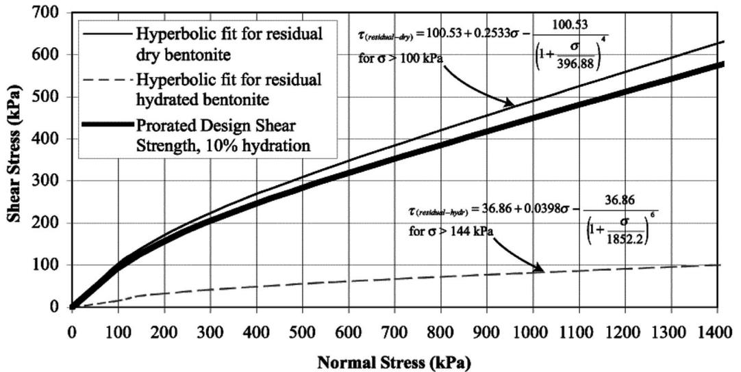
Figure 3. Prorated shear strength curve for encapsulated, partially-hydrated bentonite.
