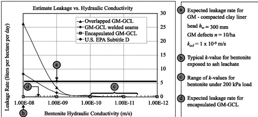
Figure 2. A comparison of hydraulic performance of example composite bottom liner systems with (a) GM-GCL alternative liners, and (b) U.S. EPA subtitle D composite bottom liner.
