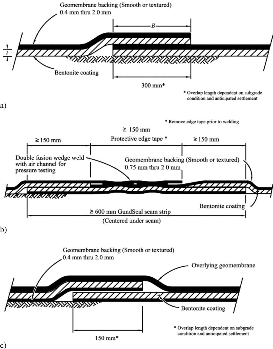
Figure 1. Typical GM-GCL Installation Options. a) Overlapped GM-GCL, shingle seams. b) Double wedge fusion welded GM-GCL seams. c) Encapsulated GM-GCL.
