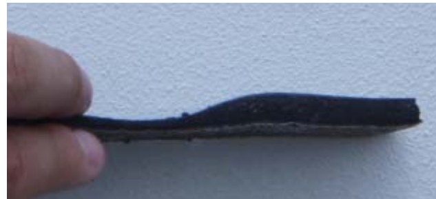
(f) Gasket that was under an overlapped batten showing a section that was crushed past its elastic limit, and a section that was not compressed.
