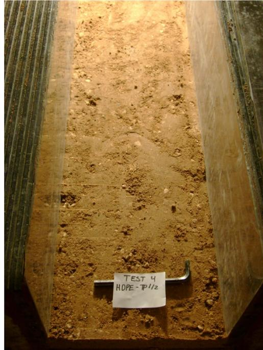
Figure 2. Typical surface of subgrade soil prior to placement of geomembrane.
