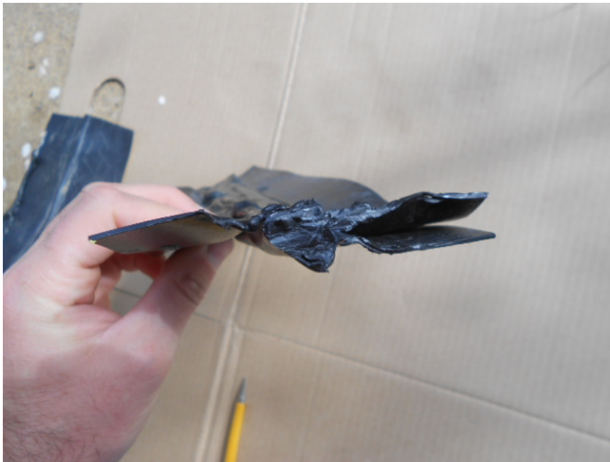
...view from side showing extreme overheating.
