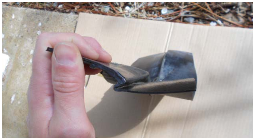
Bottom side of overheated extrusion weld.
