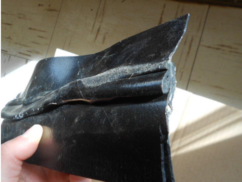
View of severely overheated extrusion weld from below.
