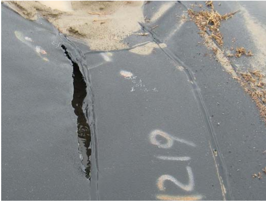
Tear in lower sheet that propagated months later.
