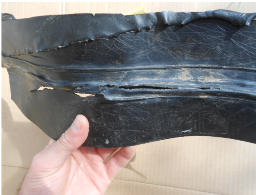
View of cracked extrusion weld.
