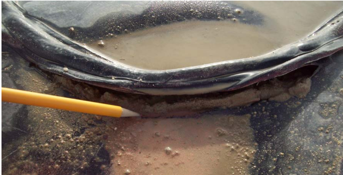
Extrusion weld cracks open after a week of exposure – it is a tear in the lower sheet that has been severely thinned.
